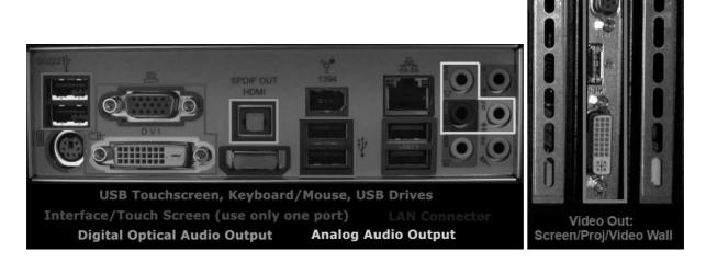
If the devices you are plugging into the dCine unit can use both analog and digital cables, as a general rule use the digital cables as opposed to analog. For example, if your projector has the choice of D-Sub (the blue trapezium shaped plugs AKA VGA) or DVI (the white plug with many pins), use the DVI cable. Similarly if your sound processor supports optical SPDIF and Analog inputs, choose the optical SPDIF connector as it will provide cleaner, higher quality sound.
